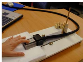
Figure 1. A specially constructed “tilt board” was used with the thermode placed at one side and weights at the other side of the board. The subject was told to keep the board in a horizontal position with his finger. By changing the weights on the opposite side of the board following pressures could be received: 200g, 400g and 600g. The measurement order was randomized.
