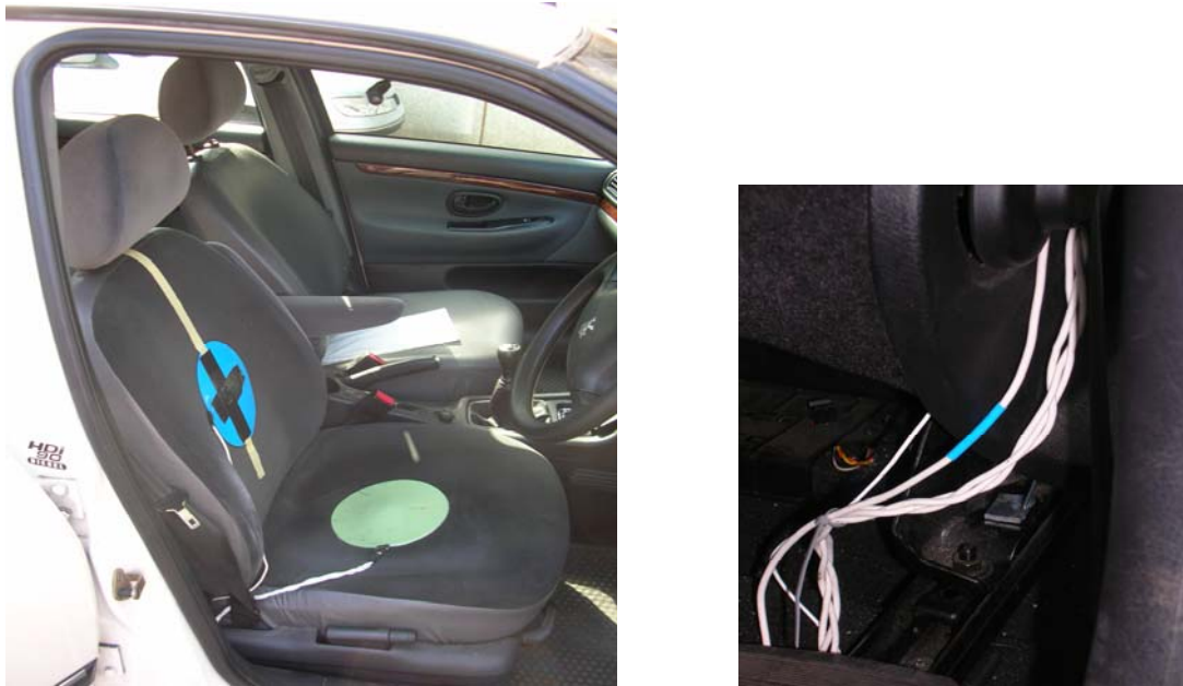
Figure 2. Measurement system (placement of SIT pad on the driver's seat)
