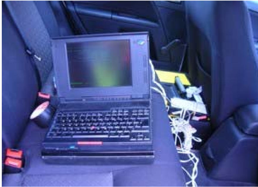
Figure 3. Measurement system (portable digital computer-based data acquisition and analysing system, HVLab (version 3.81) and 12-volt rechargeable battery
