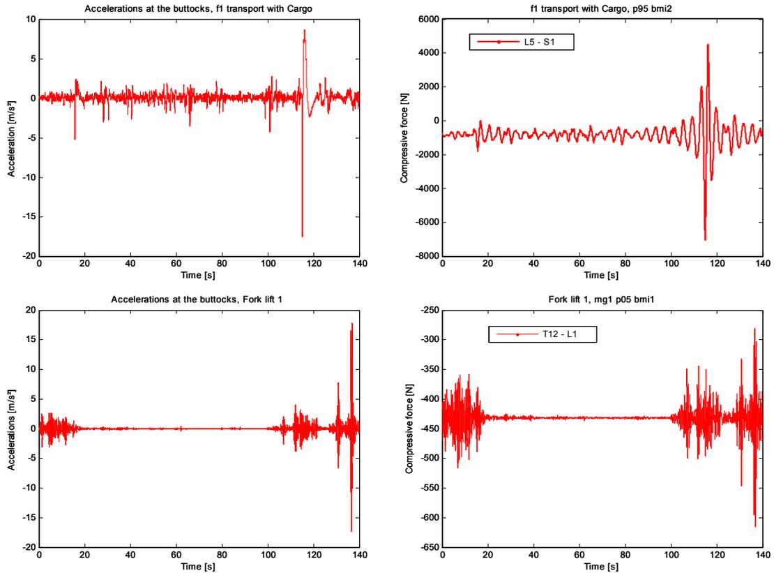
Figure 7. Input accelerations in z-axis (left) and the resulting compressive forces (sum of static and dynamic forces) with the maximum number of peak-to-peak values (bottom, right) and with the highest maximum peak-to-peak value (top, right). The insets designate the exposure condition/posture (cf. Table 3), the percentile of body mass (p), the body mass index (bmi) (cf. Annex to report on WP6, task 6.1) and the disc level.
