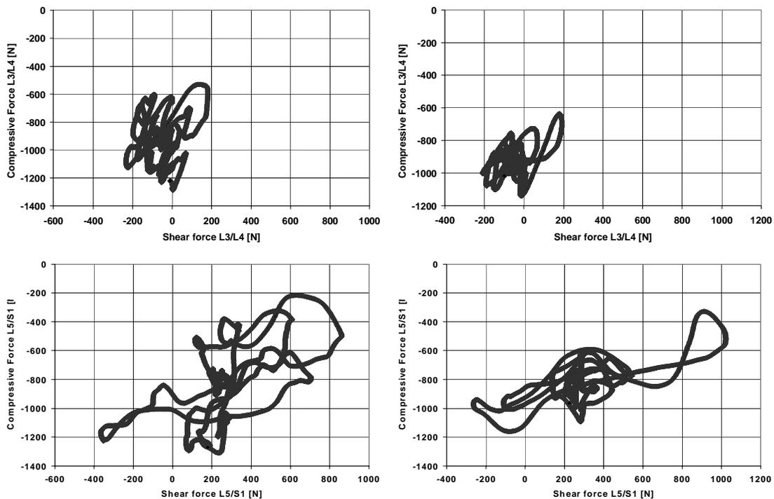
Figure 19. Bidimensional plots of predicted (driver with BMI2, body mass of P95) shear forces in x-direction and compressive forces acting on the disc L3/L4 (top) and L5/S1 (bottom) during two different segments (left and right) of the exposure "Forwarder1 Transport no Cargo" (cf. Table 3). Static and dynamic forces were summed up. Compression = negative sign, ventral shear of the upper vertebra = positive sign.
