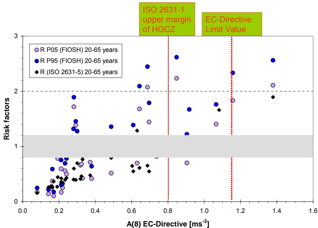
Figure 23. Comparison of risk assessments for exposure conditions listed in Table 3, R P05 and R P95 – risk factors described in Section 1.1, calculated for an ultimate strength of the 50<sup>th</sup> percentile and the lumbar level L4/L5, R – factor defined in ISO 2631-5 without specification of posture, anthropometric characteristics and disc level. P05 – body mass of the 5<sup>th</sup> percentile and BMI1, P95 – body mass of the 95 percentile and BMI2. HGCZ – health guidance caution zone.
