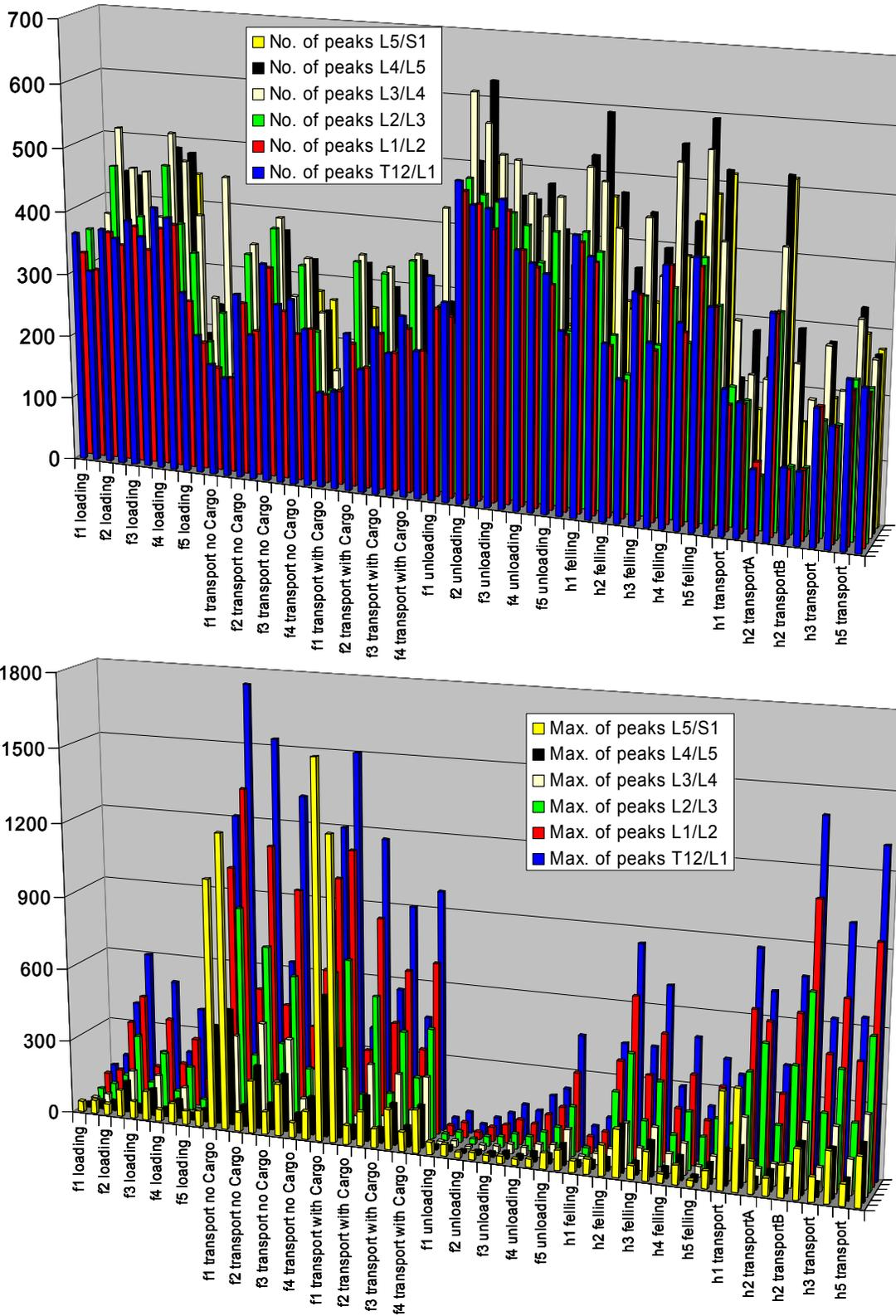
Figure 15. Number (top) and maxima (bottom) of the peak-to-peak values of the lateral shear forces [N] calculated for different tasks of forestry machines (UMUH), alternately - within each task - for statures p05bmi1 (left) and p95bmi2 (right).
