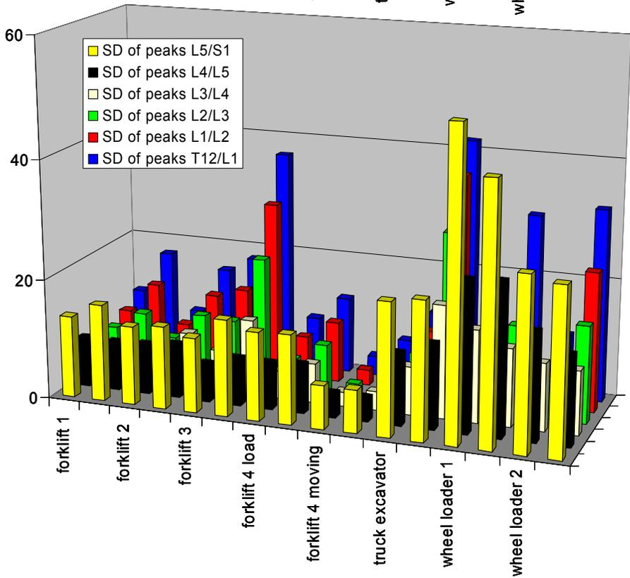
Figure 13. Mean values (top) and Standard deviations (bottom) in Newton of positive peak values of the fore-and-aft shear forces [N] calculated for different tasks of fork lifts, wheel loaders and a truck excavator, alternately for statures p05bmi1 (left) and p95bmi2 (right).
