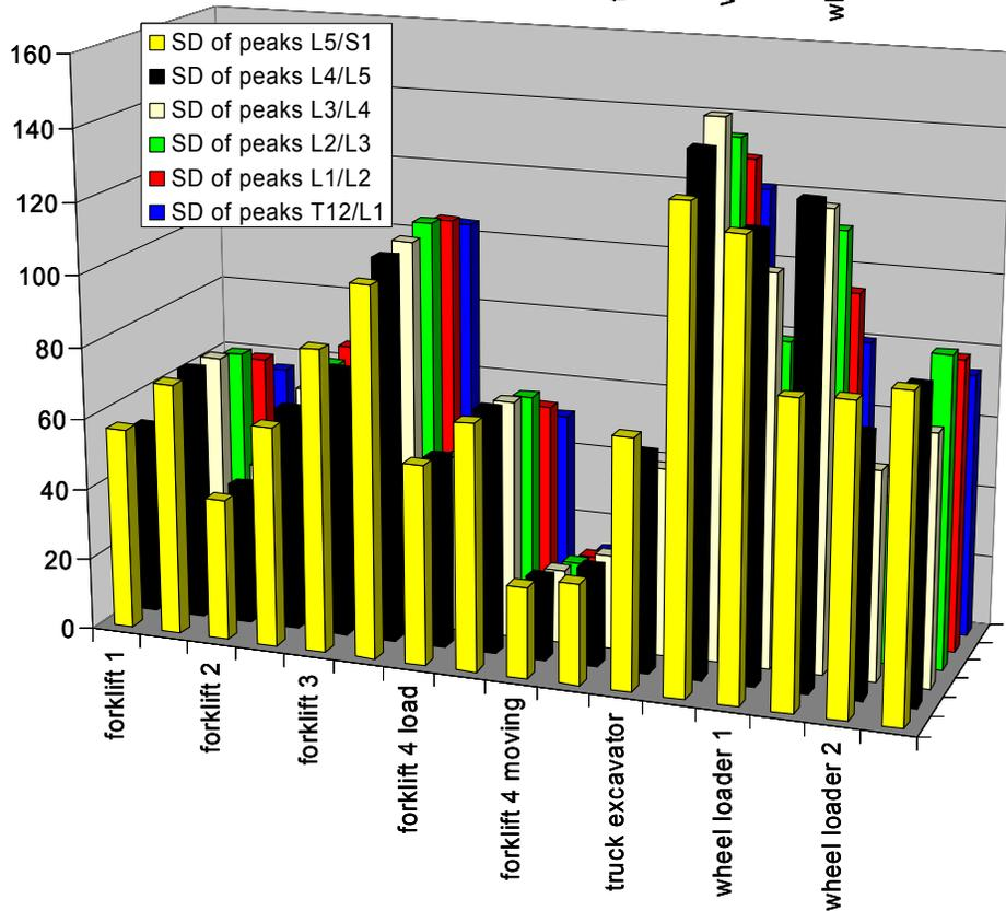
Figure 6. Mean values (top) and standard deviations (bottom) of peak-to-peak values of the compressive forces [N] calculated for fork lifts, wheel loader and a truck excavator, alternately within each machine for stature p05bmi1 (left) and p95bmi2 (right).
