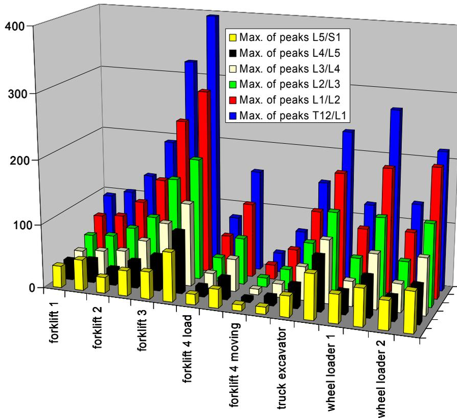
Figure 17. Number (top) and maxima (bottom) of peak-to-peak values of the lateral shear forces [N] calculated for different tasks of fork lifts, wheel loaders and a truck excavator. alternately - within each combination of machine and task - .for statures p05bmi1 (left) and p95bmi2 (right)
