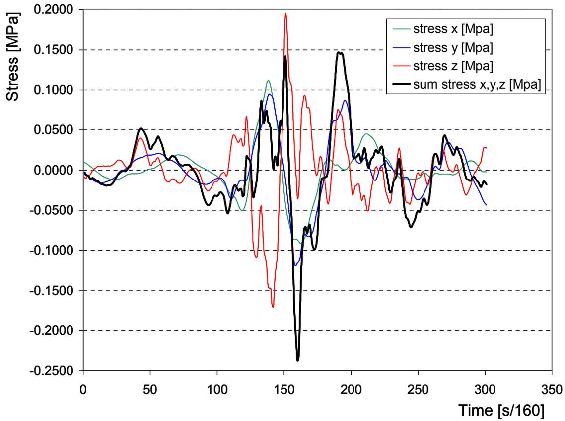
Figure 24. Small portion of predicted components of the compressive stress according to ISO 2631-5 (2004) due to spinal responses in x-, y-, and z-axis together with the sum of compressive stress. Exposure condition – WL1, 116.236 – 118.112 s from the beginning of the time series.
