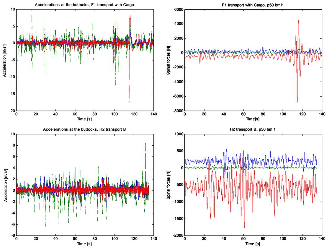
Figure 20. Input accelerations (left) and spinal forces (right, calculated for the 50<sup>th</sup> percentile and BMI1)) for the condition 'Forwarder 1 transport with Cargo' (top) and 'Harvester 5 transport B' (bottom) for a duration of 140 (blue- x-direction, green – y-direction, red – z-direction).
