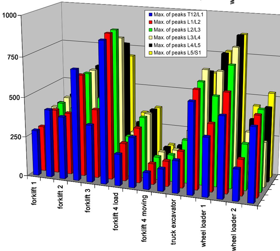
Figure 5. Number (top) and maxima (bottom) of peak-to-peak values of the compressive forces [N] calculated for fork lifts, wheel loaders and a truck excavator (Trieste), alternately within each machine for statures p05bmi1 (left) and p95 bmi2 (right).
