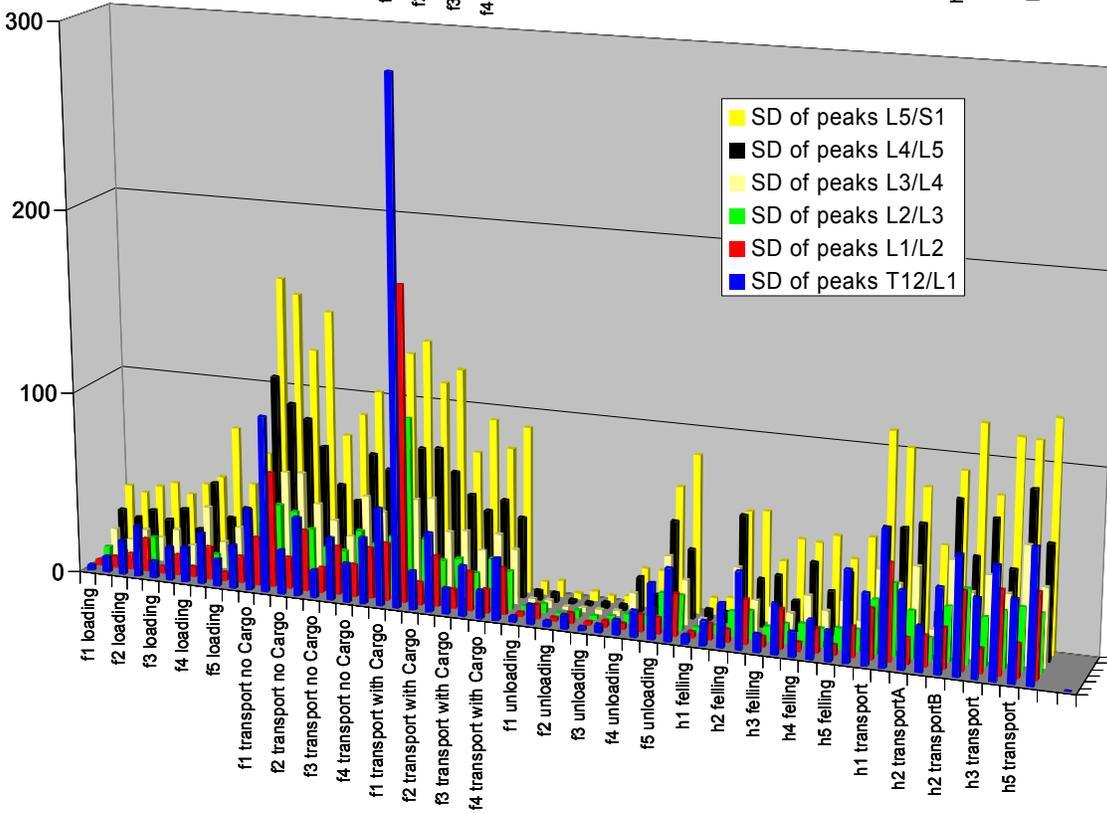
Figure 11. Mean values (top) and Standard deviations (bottom) of the positive peak values of the fore-and-aft forces [N] calculated for different tasks forestry machines (UMUH), alternately - within each task - for statures p05bmi1 (left) and p95bmi2 (right).
