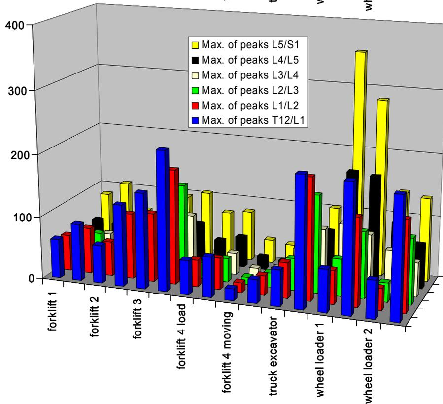
Figure 12. Number (top) and maxima (bottom) of positive peak values of the fore-and-aft shear forces [N] calculated for different tasks of fork lifts, wheel loaders and a truck excavator, alternately - within each combination of machine and task - for statures p05bmi1 (left) and p95bmi2 (right)
