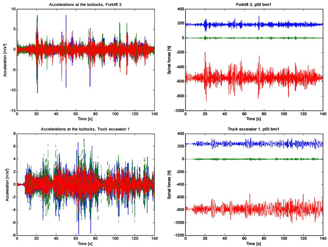
Figure 22. Input accelerations (left) and spinal forces (right, calculated for the 50<sup>th</sup> percentile and BMI1) for the condition 'Forklift 3' (top) and 'Truck excavator' (bottom) for a duration of 140 (blue- x-direction, green – y-direction, red – z-direction).
