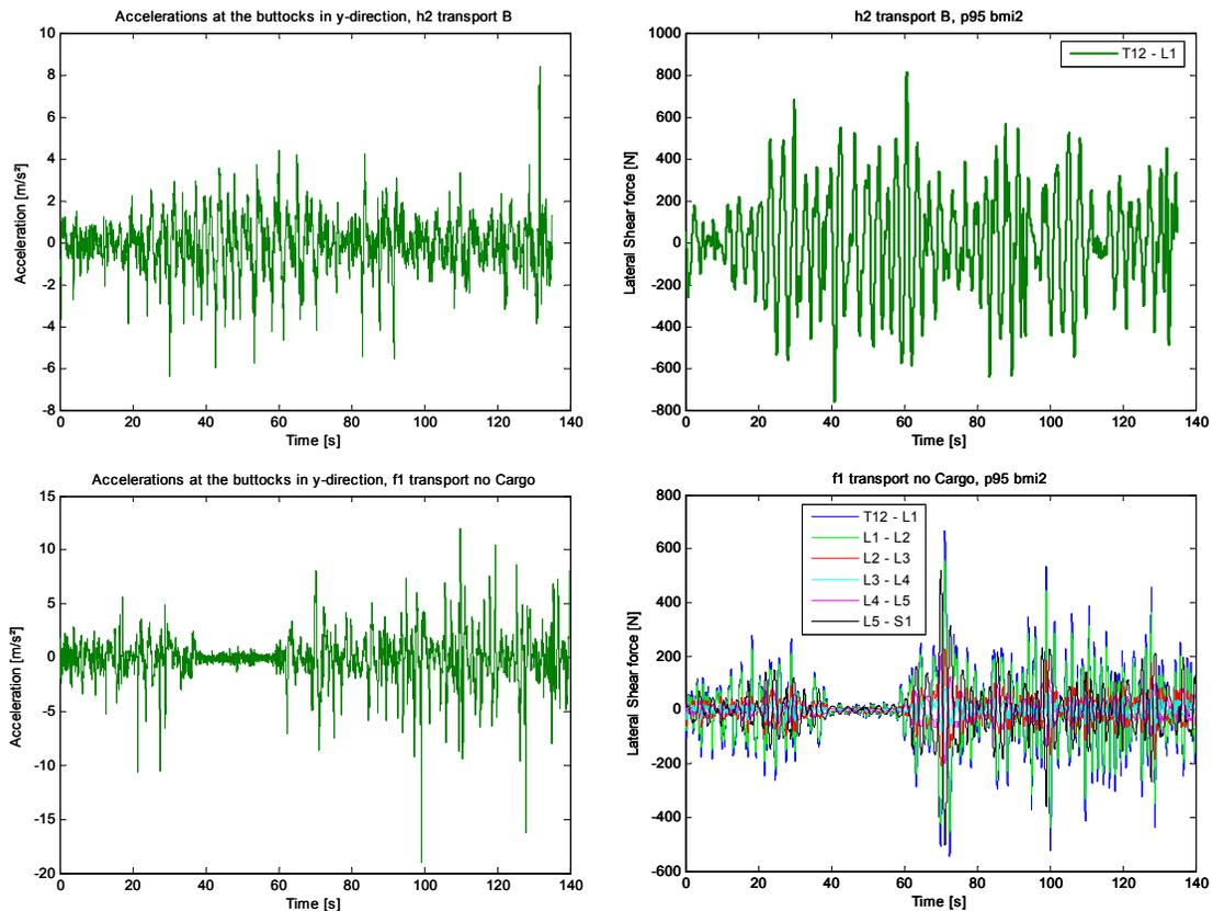
Figure 14. Input accelerations (left) and resulting lateral shear forces (right) with the highest mean value and standard deviation (top) and with the highest peak-to-peak values (bottom).
