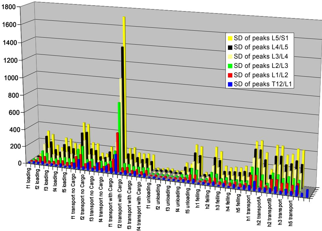
Figure 4. Mean values (top) and Standard deviations (bottom) of peak-to-peak values of the compressive forces [N] calculated for different tasks of forestry machines (UMUH) and - alternately within each task - for statures p05bmi1 (left) and p95 bmi2 (right).
