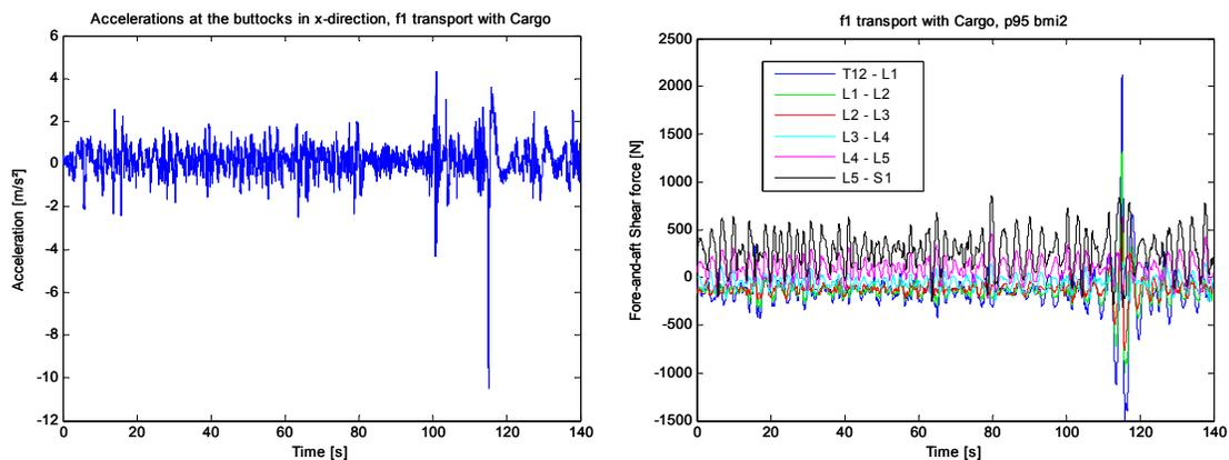
Figure 9. Input acceleration in the fore-and-aft direction measured at the seat (left) and the calculated fore-and-aft shear forces (sum of static and dynamic shares) at six spinal levels.
