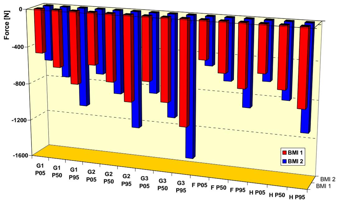
Figure 1. Static compressive forces (in N) predicted for the level L4/L5 caused by different postures (G1...G3, F-forwarder, H-harvester) and anthropometric characteristics of different percentiles (P) of European drivers with a body mass index  $\leq 2.6122 \text{ g/cm}^2$  (BMI 1) or  $> 2.6122 \text{ g/cm}^2$  (BMI 2).
