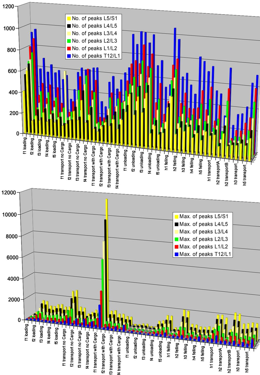
Figure 3. Number (top) and maxima (bottom) of peak-to-peak values of the compressive forces [N] calculated for different tasks of forestry machines (UMUH) and - alternately within each task - for statures p05bmi1 (left) and p95 bmi2 (right).
