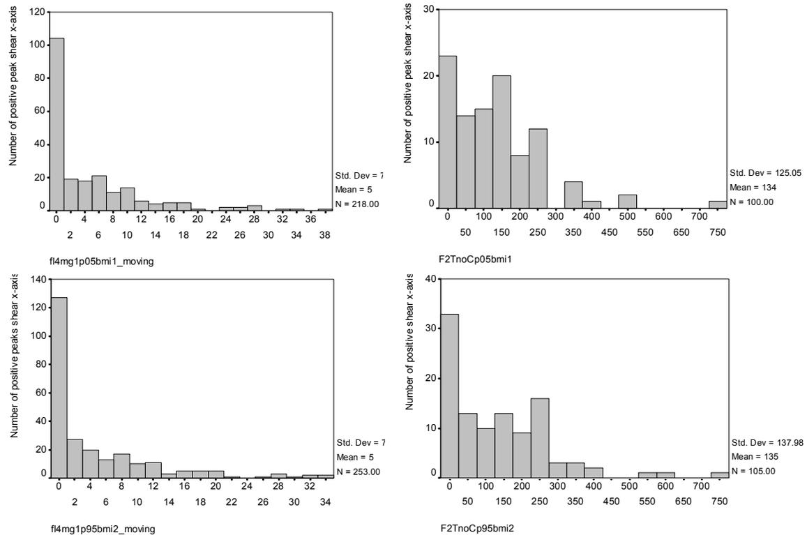
Figure 8. Histograms of peak dynamic positive (forwards) shear forces in [N] (x-axis) calculated for disc L5/S1 during exposures on forklift 4 moving paper mills (left) and on forwarder 2, transport no cargo (cf. Table 3) for a driver of the 5<sup>th</sup> percentile with a body mass index  $\leq 2.61 \text{ g/cm}^2$  (top) (cf. Report on WP 6, Task 6.1) and driver of the 95<sup>th</sup> percentile with a body mass index  $> 2.61 \text{ g/cm}^2$  (bottom) (cf. Annex to Report on WP 6. Task 6.1)
