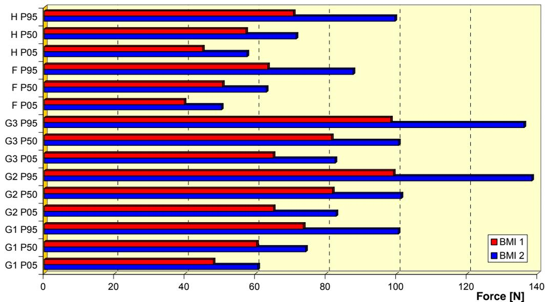
Figure 2. Static shear forces (in N) predicted for the level L4/L5 caused by different postures (G1...G3, F-forwarder, H-harvester) and anthropometric characteristics of different percentiles (P) of European drivers with a body mass index  $\leq 2.6122 \text{ g/cm}^2$  (BMI 1) or  $> 2.6122 \text{ g/cm}^2$  (BMI 2).
