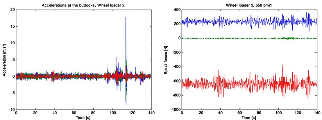
Figure 21. Input accelerations (left) and spinal forces (right, calculated for the 50<sup>th</sup> percentile and BMI1)) for the condition 'Wheel loader 2' for a duration of 140 (blue- x-direction, green – y-direction, red – z-direction).
