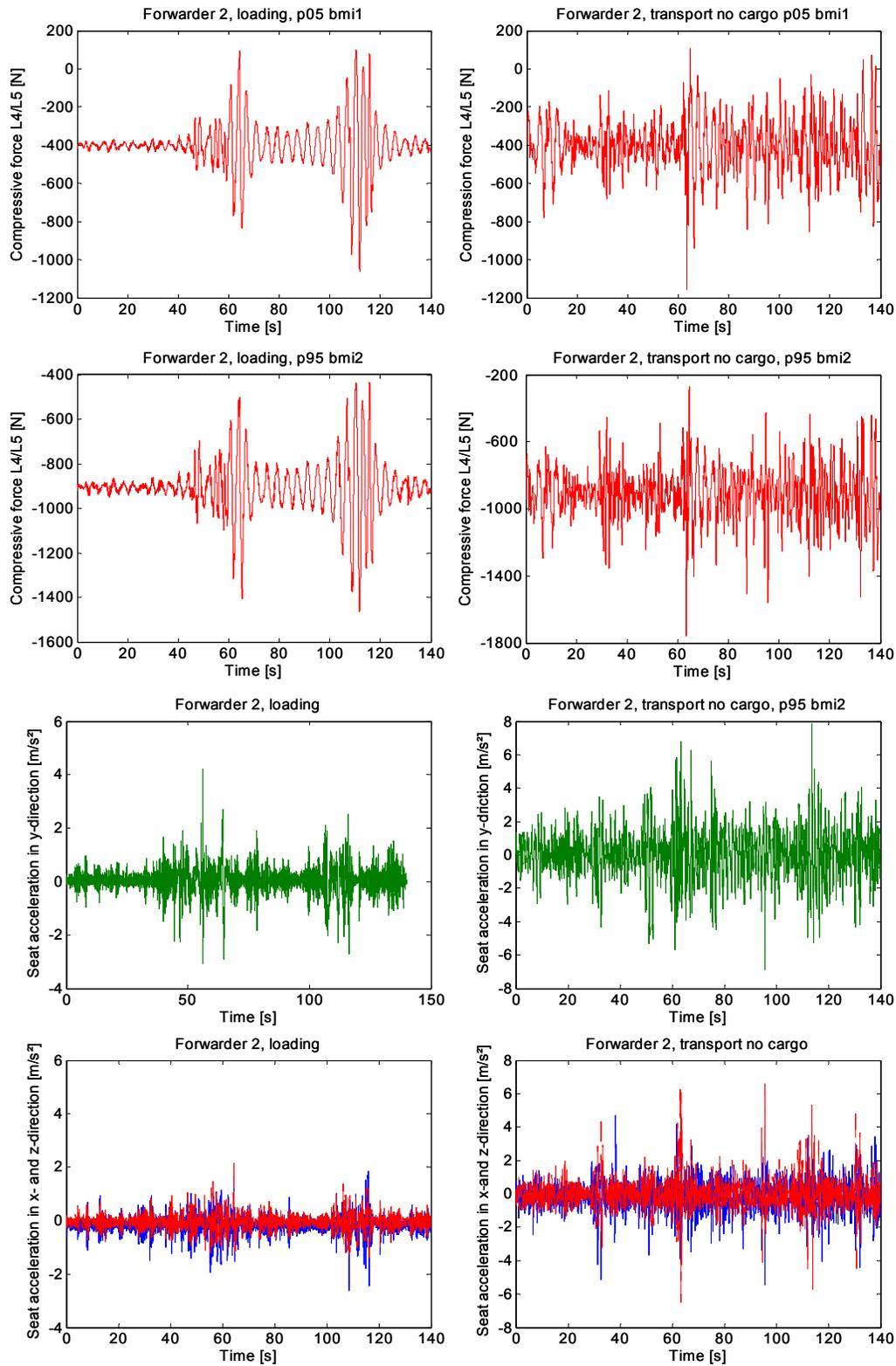
Figure 25. Predicted compressive forces acting on L4/L5 during seat accelerations in x-, y- and z-directions. p – percentile of body mass, bmi – body mass index. See text for details.
