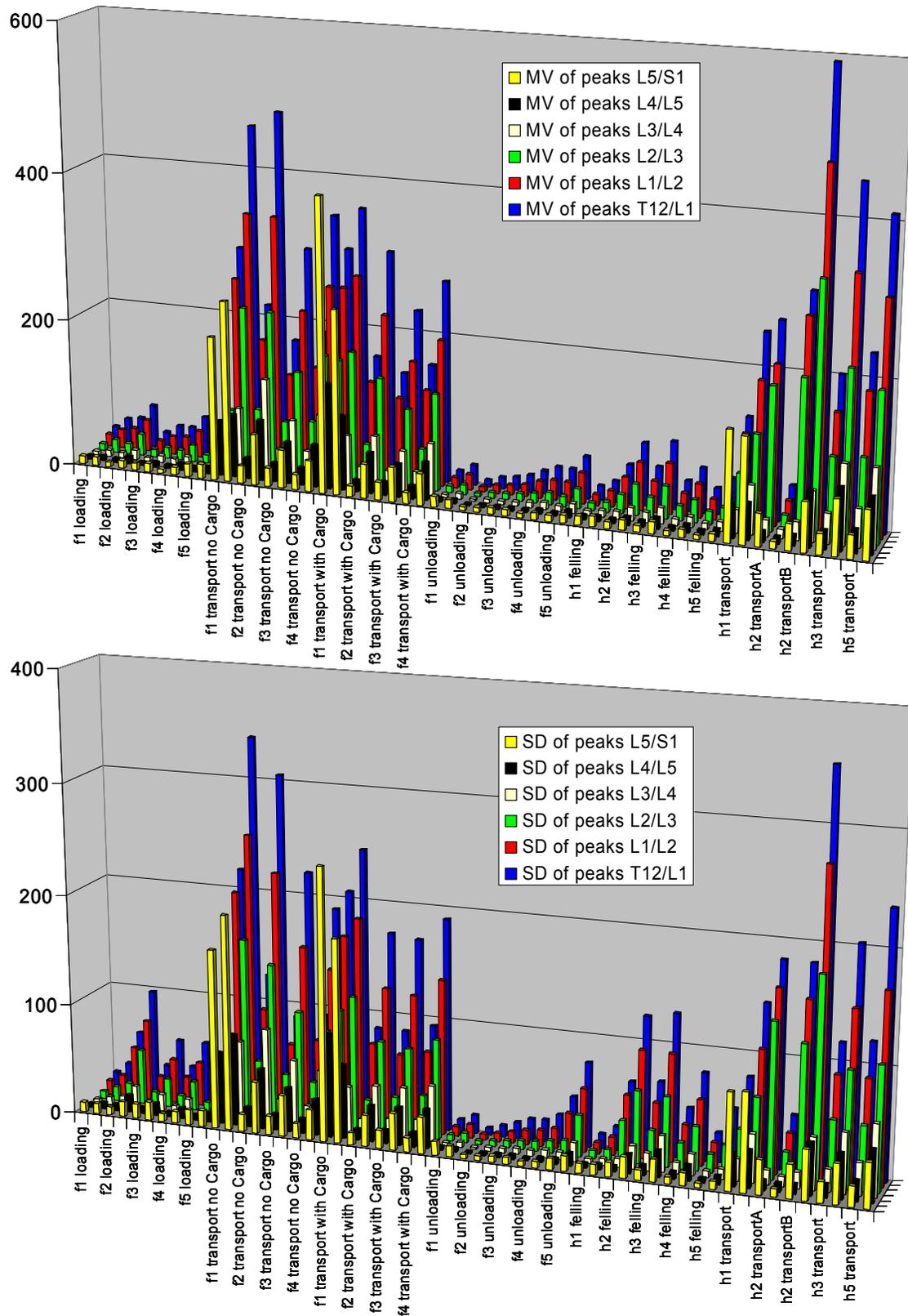
Figure 16. Mean values (top) and Standard deviations (SD, bottom) of the peak-to-peak values of the lateral shear forces [N] calculated for different tasks of forestry machines (UMUH), alternately - within each task - for statures p05bmi1 (left) and p95bmi2 (right).
